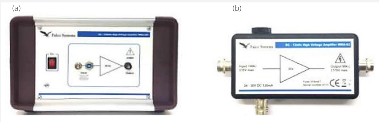
Figure 2. Photographs of 2 types of amplifier for HV measurements (a) type 1 and (b) type 2.
