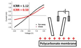
Ion current rectification measurements of surfaces with Park XE-Bio. By measuring the current-voltage rectification response (ICRR) far away from a surface and close to a surface, the net surface charge can be deduced. In plots shown a positive surface charge is measured for a solution of lithium ions in propylene carbonate.
