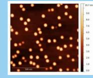
AFM image demonstrating the 1×1 1×1 micron area used for the dot statistic. - See more at: http://lnnano.cnpem.br/ laboratories/mta/thin-film-growthfacilities/#sthash.cPDISisF.dpuf
