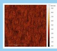
10×10 micron AFM image of InAs self-assembled islands grown at ca. 500°C.
