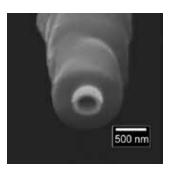
A hybrid scanning electrochemical microscopy – scanning ion conductance microscopy (SECM-SICM) probe. The central barrel is used for SICM and provides distance control, the crescent-shaped gold electrode is used to measure faradaic electron transfer. The entire pipette is insulated in a layer of vapor-deposited parylene.
