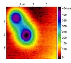
Image collected by Scanning Electrospray Microscopy (SESM) module develop with the Park XE-Bio. Two one micron polystyrene particles can be observed, where electrospray from a nanopipette provided feedback and position control.
