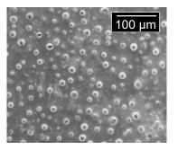
This image shows a Nafion© membrane that has been chemically degraded. With SICM-SECM, changes in ion transport through the degraded membrane were observed.
