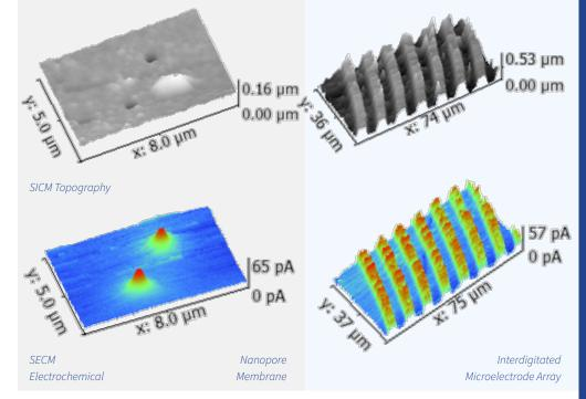
(Bottom) Scanning electrochemical microscopy (SECM) is used to meaure diffusion of redox active molecules through the nanopores of the membrane or to measure redox cycling at the microelectrode array.
