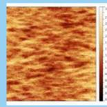
10×10 micron AFM image of a hydrogen cleaned substrate surface with 10 ML of GaAs redeposited after cleaning.
