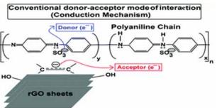
hydrogen bonding between rGO and PANI, which provide a route for constructing highly ordered chain structures with improved thermoelectric performance of PANI. There is no significant change in the thermal conductivity of the rGO–PANI composite as compared to pure PANI, which improves the thermoelectric performance of composite.
