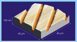
First atomic force microscope image on Mars. This calibration image presents three-dimensional data from the atomic force microscope on NASA's Phoenix Mars Lander, showing surface details of a substrate on the microscope station's sample wheel. It will be used as an aid for interpreting later images that will show shapes of minuscule Martian soil particles. Image NASA/JPL-Caltech/University of Arizona/University of Neuchatel
