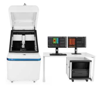
Figure 4. Atomic force microscopy system (Courtesy Park Systems Inc).
