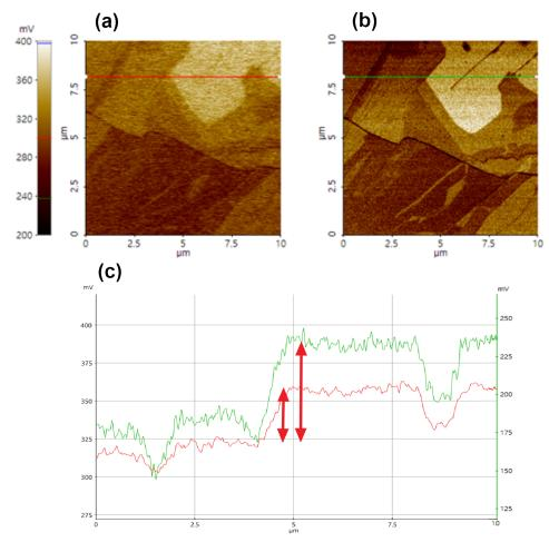
Figure 3. The comparison of surface potential between AM-KPFM (a) and Sideband KPFM (b) on a HOPG sample with a line profile analysis (c).
