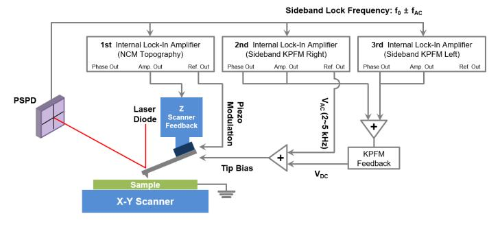
Figure 2. Connection diagram of Sideband KPFM.
