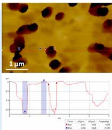
Figure 4. Topography images of 400nm diameter pore polycarbonate membrane recorded in PBS solution with SICM ARS mode. The average pore depth is ~ 600nm.
