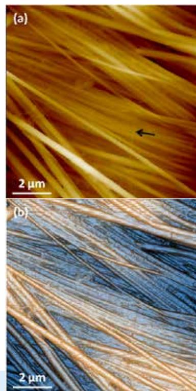
Figure 5. (a) Topography and (b) contrast enhanced topography images of collagen sample imaged in PBS solution with SICM ARS mode. Individual fibril can be clearly identified and the thinnest one observed is about 90nm in width, as pointed by the black arrow. Scan size 10μm×10μm. Image size 256 px× 256 px.
