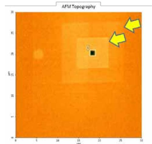
Figure 8. AFM image of a Facet defect with several SEM burn-marks is shown. The SEM burn-marks are marked by arrows.
