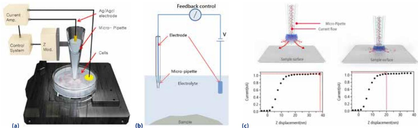
Figure 1. The snapshots showing the (a) SICM hardware setup, (b) circuit mechanism and (c) current-distance relationship between the pipette end and the sample surface.
