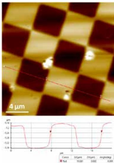
Figure 2. Topography image of the XY standard sample acquired by DC mode. Scan size 20μm×20μm. Image size 215 px× 215 px.
