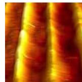
*Nanopatterned lines on a precursor polymer thin film Nanoscale smart coating features such as these patterned lines can be imaged using a conductive AFM setup.*
