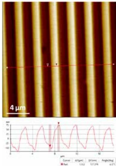
Figure 3. Topography image of the XY standard sample acquired by DC mode. Scan size 20μm×20μm. Image size 256 px × 256 px.
