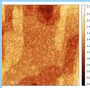
AFM Image of the surface of a AlGaAs/GaAs heterostructure.
