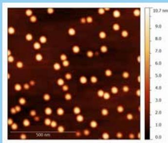
AFM image demonstrating the 1×1 1×1 micron area used for the dot statistic. - See more at: <http://lnnano.cnpem.br/laboratories/mta/thin-film-growth-facilities/#sthash.cPDISisF.dpuf>
