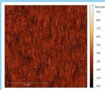
10×10 micron AFM image of InAs self-assembled islands grown at ca. 500°C.
