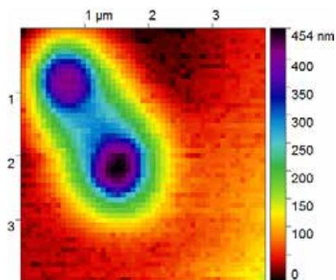
Image collected by Scanning Electro Spray Microscopy (SESM) module developed with the Park XE-Bio. Two one micron polystyrene particles can be observed, where electro spray from a nanopipette provided feedback and position control.
