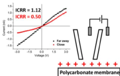
Ion current rectification measurements of surfaces with Park XE-Bio. By measuring the current-voltage rectification response (ICRR) far away from a surface and close to a surface, the net surface charge can be deduced. In plots shown a positive surface charge is measured for a solution of lithium ions in propylene carbonate.
