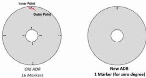
Figure 4. The schematic shows the sample alignment process in the first (left) versus the new (right) generation of Park ADR-AFM. In the latest Park ADR-AFM only one marker is needed to indicate zero-degree location of hard disk media samples.
