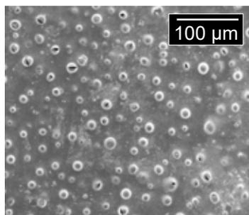
This image shows a Nafion<sup>®</sup> membrane that has been chemically degraded. With SICM-SECM, changes in ion transport through the degraded membrane were observed.
