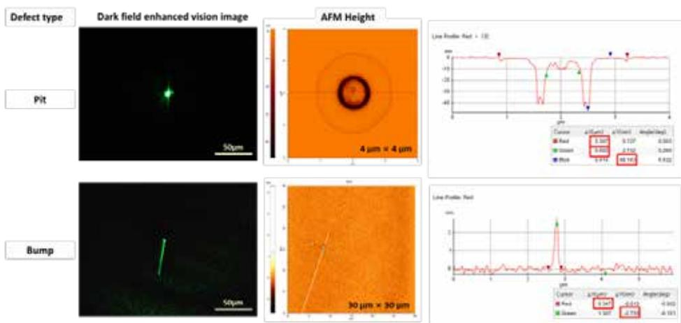
Figure 7. Representative pit and bump type defects on a hard disk media samples which were found and imaged by ADR-AFM. The dark field enhanced vision images are shown side by side the AFM images and selected profiles of the defects.
