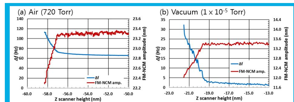
Figure 6 -  $\Delta f$ -distance curve in a narrow Z scanner height range (10nm) about (a) air and (b) vacuum condition.
