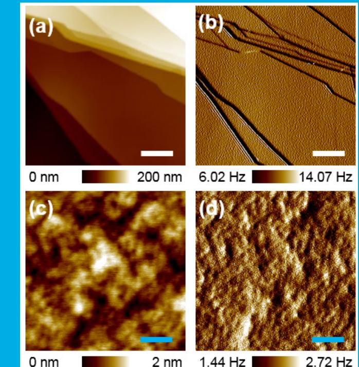
Figure 8 - FM-NC-AFM image in vacuum condition. HOPG (a) topography and (b) error signal( $\Delta f$ ). White bar is 2  $\mu\text{m}$ . Silicon (c) topography and (d) error signal( $\Delta f$ ). Blue bar is 40 nm.
