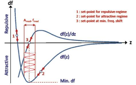
Figure 3 - A representative frequency shift-distance curve. The forces reflect the Lennard-Jones potential for sample-tip interactions.
