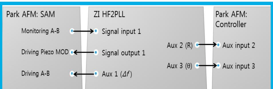
Figure 5 - Setup BNC connections: Park NX-Hivac with the four inputs for recording and controlling of image data and the one output for input the PSPD signal to HF2PLL, HF2PLL with Signal Input 1, Signal Output 1, and the Auxiliary Outputs 1 to 3, SAM with the Vertical Output (PSPD A-B signal), the input for the piezo modulation and the change in frequency due to the interaction between the sample and tip.
