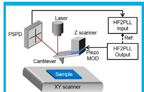
Figure 4 - AFM diagram for NC-AFM. A cantilever is brought into frequency/amplitude feedback and modulated by a piezo modulation (MOD). The vertical and lateral cantilever movement is detected by a PSPD using laser reflection on the cantilever.
