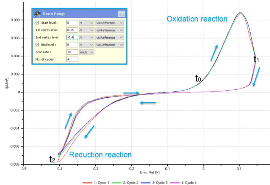
Figure 2. Cyclic voltammograms. The negative peaks demonstrate the reduction reaction state where copper is deposited in the sample. While the positive peaks demonstrate the oxidation reaction state where copper is dissolved in the sample.
