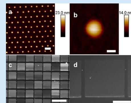
(a) AFM of a dot array with a 190 nm pitch in a hexagonal pattern array written using hard transparent array, 200 nm scale bar; (b) single polymer feature with a circle of small droplets from original meniscus, 20 nm scale bar; (c) dark-field optical microscopy of array with 500 nm pitch written using hard transparent array with PPL with 14 641 features written per pen, 100 µm scale bar; and (d) zoomed in image pattern made from a single pyramidal pen, 25 µm scale bar.
