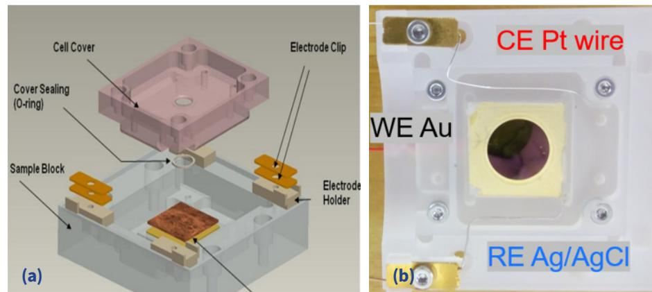
Figure 1. (a) Overall structure of the NX EC Cell (b) Actual setup of EC cell
