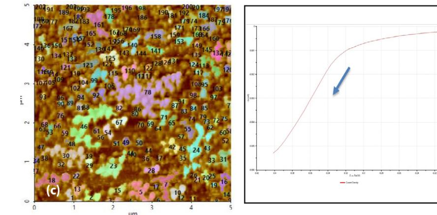
Figure 4 - (a) and (c) AFM images acquired on 1st and 2nd deposition test, (b) and (d) CV curves acquired using linear sweep voltammetry with voltages from -0.2V to -0.4V on 1st and 2nd deposition test.
