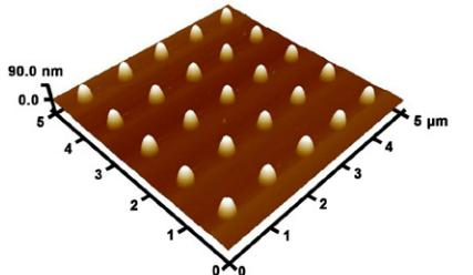
*Photo Caption: AFM topographical image of a polymer dot array printed by dip-pen nanolithography*
