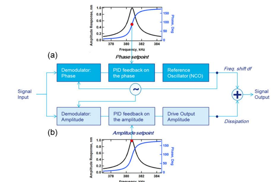
Figure 2 - Feedback loop where (a) FM and (b) AM techniques occur at the same time using HF2PLL system.
