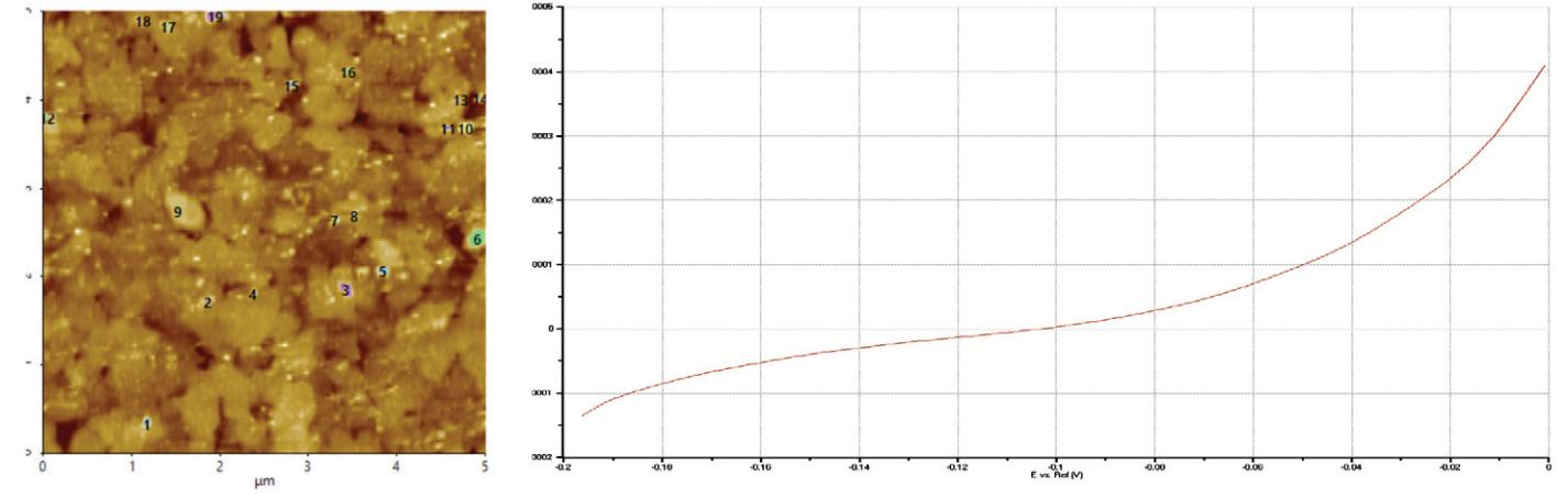
Figure 6 - (a), (c), (f), and (h) AFM images acquired on 1st to 4th dissolution test, (b), (d), (g) and (i) CV curves acquired using linear sweep voltammetry with voltages from -0.2 V to 0 V on 1st to 4th dissolution test.
