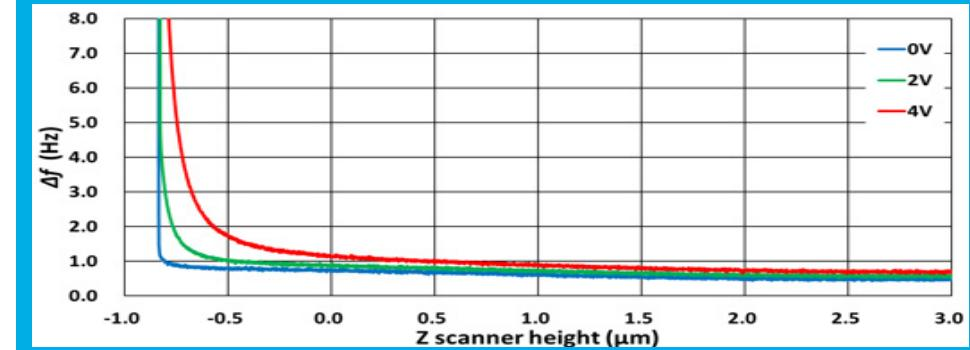
Figure 7 -  $\Delta f$ -tip bias curve in vacuum. The  $\Delta f$  value begins at 0 Hz (graph is read right to left) and when the slope of the FM-NC-AFM amplitude increases sharply, the tip has approached the surface. As the tip bias is increased from 0 to 4 V, the approach is increasingly damped and the sharp increase in  $\Delta f$  occurs further from the sample surface with increased voltage.
