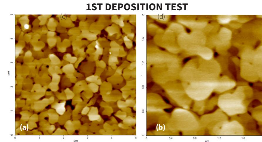
Figure 3 - (a) AFM image acquired in air, (b) AFM image acquired in liquid
