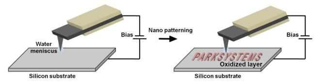
Figure 1. Schematic representation of bias-assisted AFM nanolithography via local surface oxidation. Patterns are created on the surface by oxidation upon bias application between tip and sample.
