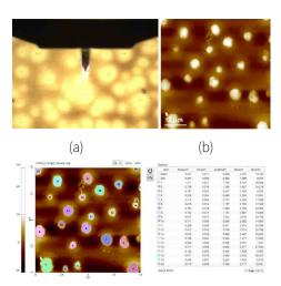
Figure 5. Optical (a) and AFM topography (b) images of the PS-LDPE copolymer standard sample as scanned using StepScan autocript mode. (c) "Grain analysis" as performed with the image processing software Park XEI based on customized criteria to determine the areas of each LDPE cluster. Scan size: 10 µm × 10 µm, image size: 256 px × 256 px.
