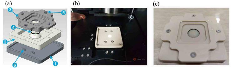
Figure 1. (a) Schematic structure of the liquid cell design for contact lenses, (1) Cell adapter for AFM body (2) Cell Base (3) Cell bracket (4) O-ring between base and bracket (5) 2 $\Phi$  bolts (6) 2.5 $\Phi$  bolts; (b) Cell adapter installed on the AFM body; (c) Cell base and bracket components connected with soft contact lens inside.
