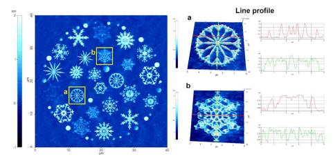
Figure 4. AFM height images after nanolithography and line profile analysis on two of the constituent structures. AFM line profiles in a and b show the ~1 nm height of the oxide layer from the substrate.
