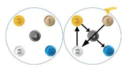
Figure 4. Diagram showing (a) the samples' distribution on the Park NX20's motorized sample stage and (b) the StepScan autocript's -created path the stage took to bring each sample to the AFM probe tip for scanning. The five samples were (1) a PS-LDPE copolymer standard sample, (2) dehydrated collagen fibrils, (3) celgard, (4) an aluminum triangular production pattern, and (5) an SRAM device.
