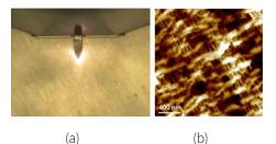
Figure 7. Optical (a) and AFM topography (b) images of the celgard sample as scanned using StepScan autoscript. Scan size: 2 µm × 2 µm, image size: 256 px × 256 px.
