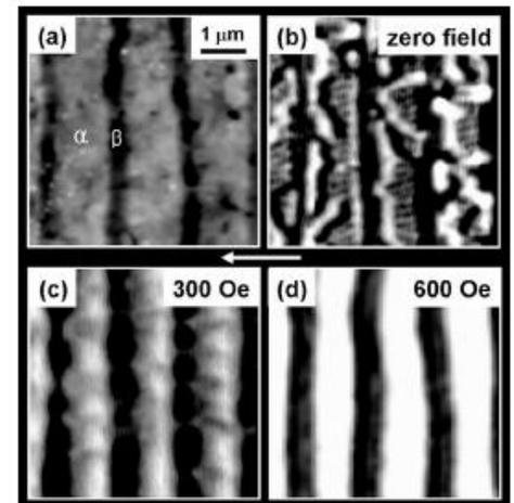
Fig. 2. (a) AFM and (b)–(d) MFM images at room temperature for 250-nm-thick MnAs film on GaAs(001). All the images were taken from the same scan area ( $5 \times 5\ \mu\text{m}$ ) and position. The magnetic field is applied along the easy axis of magnetization as indicated by the white arrow.
