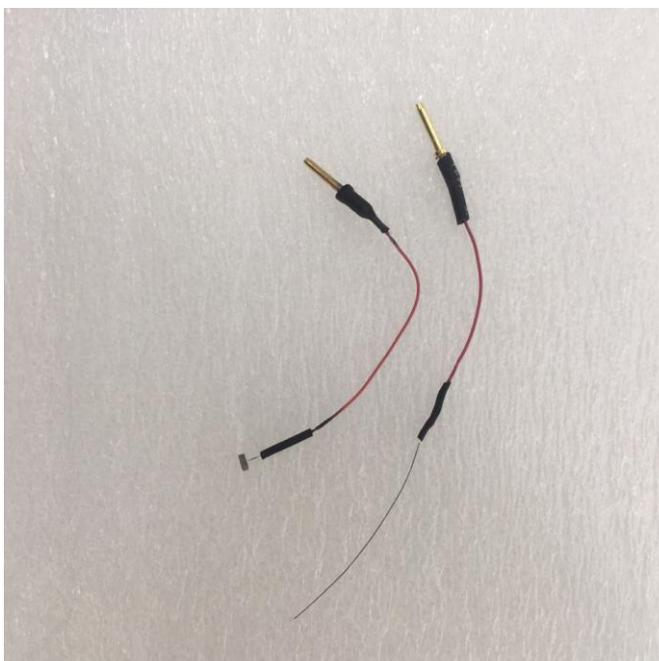
**Figure 8-5. Ag/AgCl Electrode and Nano-pipette Holder**
