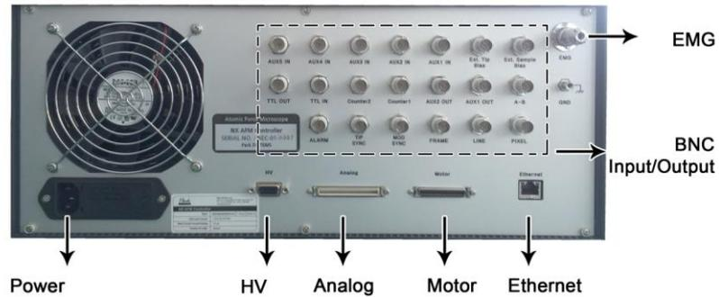
Figure 2-10. Control Electronics (Rear View)
