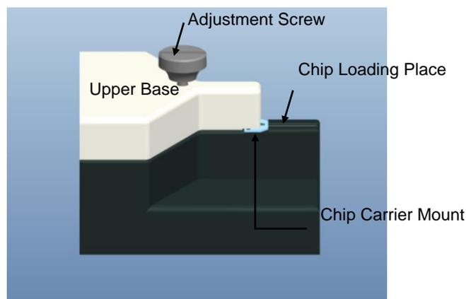
**Figure 2. Cantilever exchanger**
