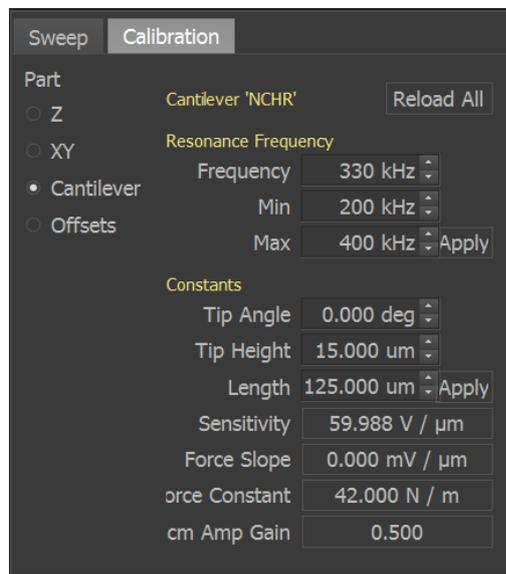
Figure A-5. Cantilever calibration setup
