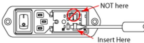
When the fuse holder is installed in the dual fuse position, it will normally release as soon as the door is opened.
