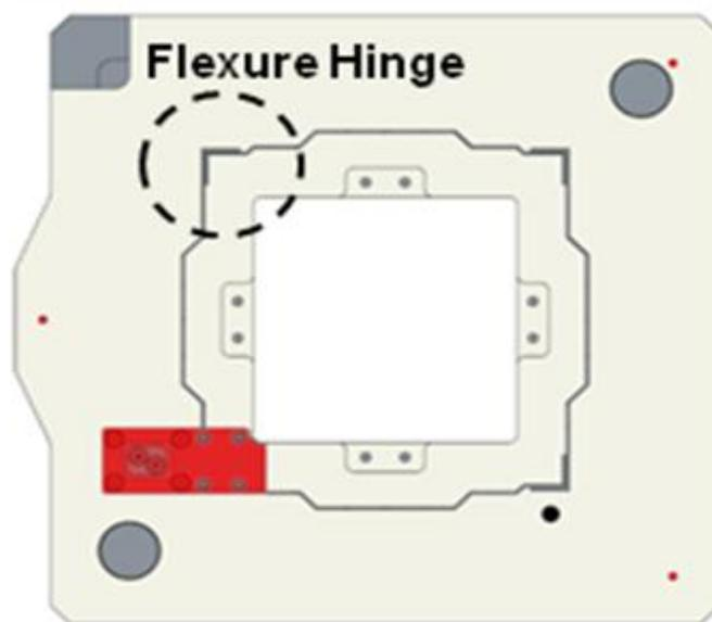
**Figure 2-7. Flexure Hinge on XY scanner**
