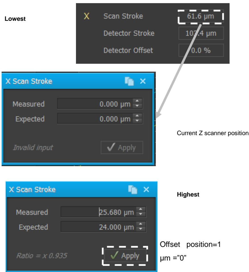
Figure A-4. XY scanner calibration example
