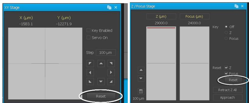
**Figure 3-16. Reset the motorized Stages**
