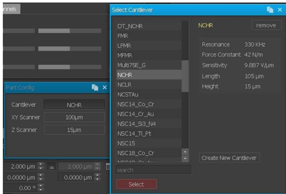
Figure 7-17. Create Cantilever DB
