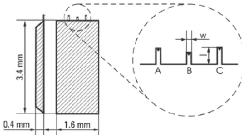
**Figure 7-22. Silicon chip of the NSC36 series has 3 rectangular cantilevers**
