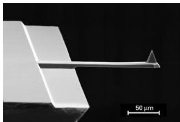
**Figure 7-9. SEM image of silicon cantilever**
