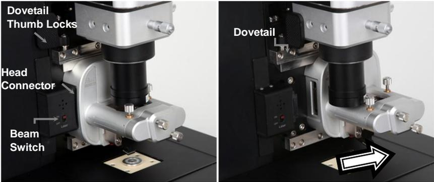
Figure 6-2. Removing NX12 Head
