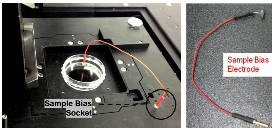
**Figure 8-14. Left: Sample Bias Socket, Right: Bias Electrode**
