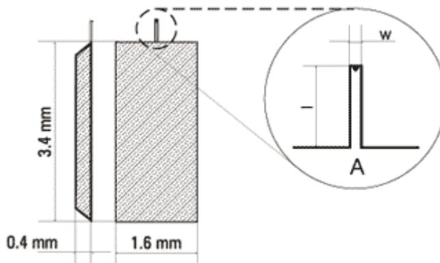
**Figure 7-33. Silicon chip of the NCHR series has 1 rectangular cantilever**
