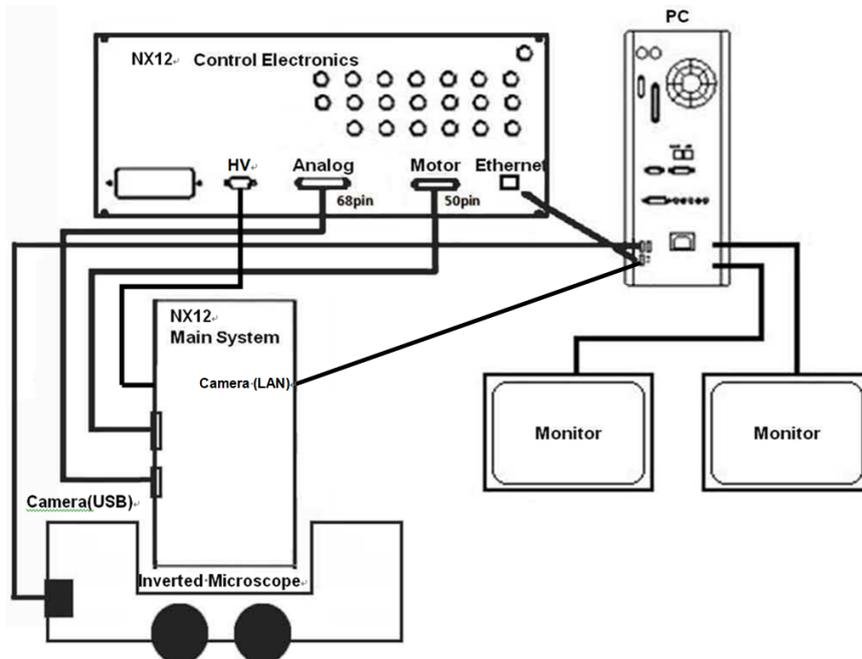
**Figure 3-14. Diagram of Cables Connections for the NX12**
