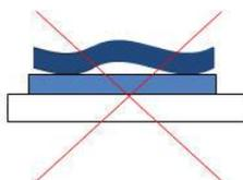
Figure 4-6. Air between Sample and Tape
