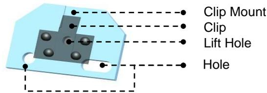
**Figure 7-15. Structure of Clip Type Chip Carrier**
