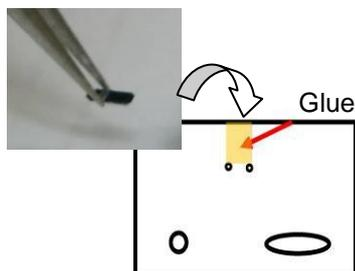
**Figure 7-12. Loading Cantilever Chip on Glue Type Chip Carrier**
