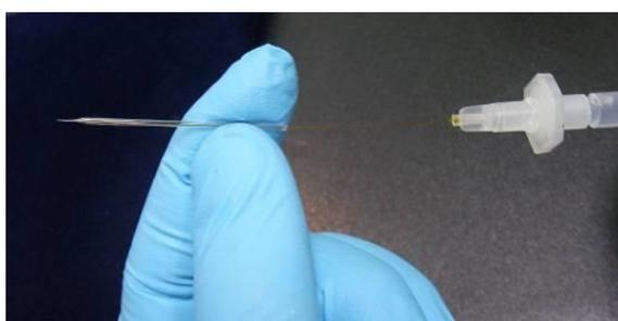
**Figure 8-4. Filling the electrolyte on the nano-pipette**
