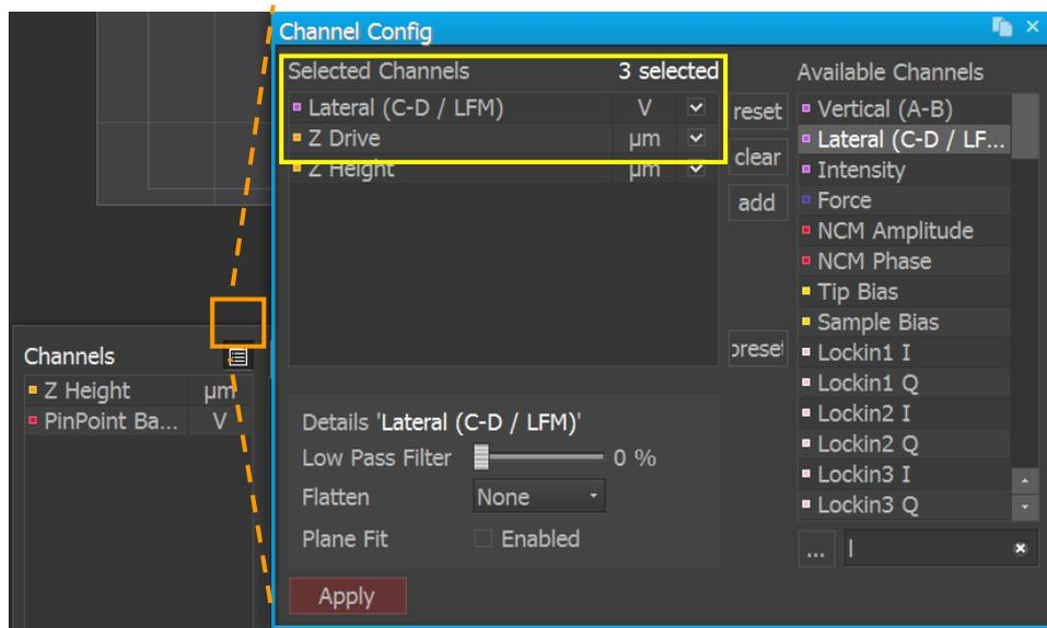
**Figure 7-27. Setup for LFM mode**
