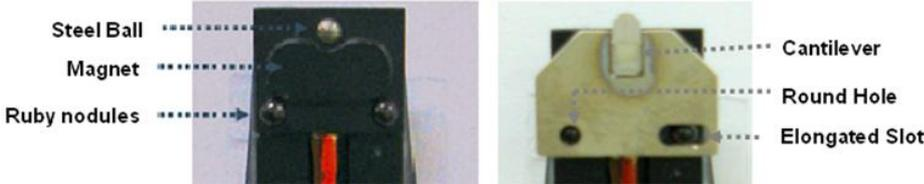
Figure 6-3. Load Cantilever onto Proband
