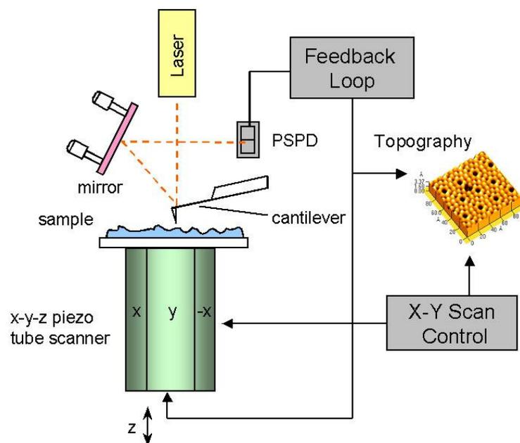
**Figure 7-1. Diagram of conventional AFM's scanning**
