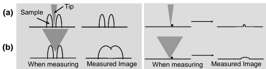
**Figure 7-10. Tip Convolution**
