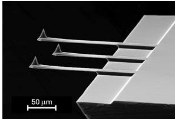
**Figure 7-21. SEM image of the shorter cantilevers (A, B, C) from a chip of the NSC36 series**
