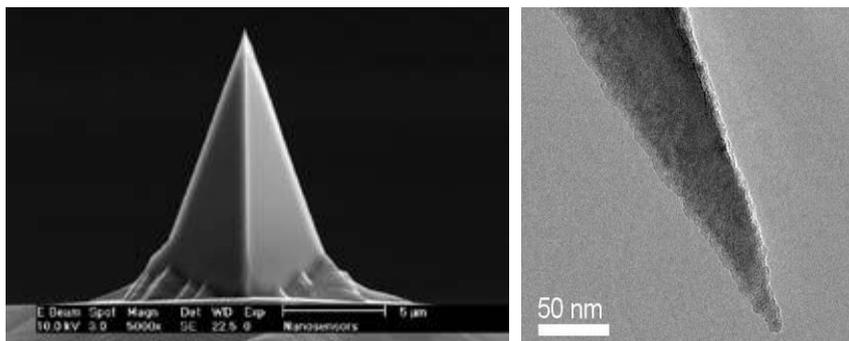
**Figure 7-32 SEM image of ULTRASHARP silicon cantilever (the PPP-NCHR series)**
