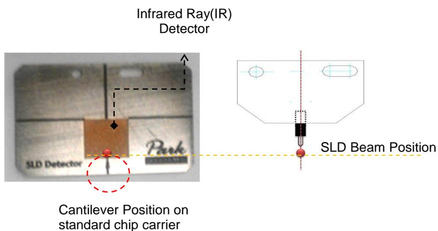
**Figure 1. (Left) Beam position when using SLD detector Chip Carrier, (Right) Beam position when using Standard Chip Carrier**
