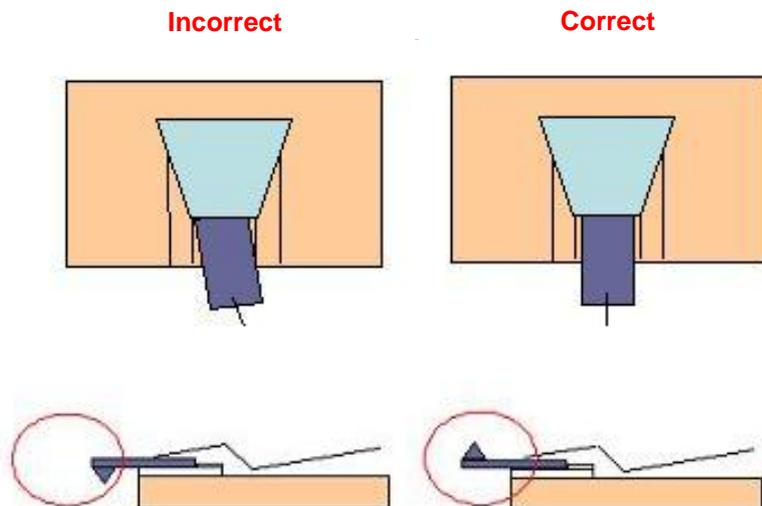
**Figure 6. Correct Mounting of Cantilever Chip**
