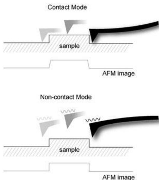
**Figure 7-28. Concept diagram of contact mode and non-contact mode**
