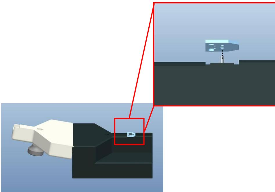
**Figure 3. Placing Clip Type Chip Carrier on Cantilever Exchanger**
