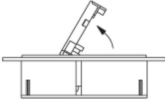
3. When the fuse holder is installed in the single fuse position, apply the screwdriver as shown and gently pry up. Insert screwdriver as shown - do not use fingers to pry the unit loose.
