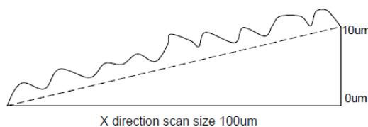
To calibrate the Z scanner, image a standard sample with a known step height and enter the measured and known (expected) heights into the calibration setup interface. A summary of the parameters for Z scanner calibration can be found in the table below. For more information about scanner calibration, please refer to the NX User's Manual.
