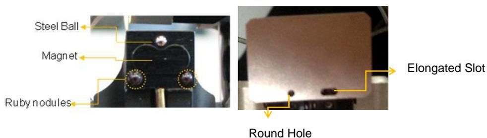
**Figure 2. (Left) Standard Probehead, (Right) with the SLD detector chip carrier attached.**
