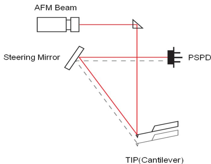
**Figure 1-5. Beam path related to the cantilever's movement**
