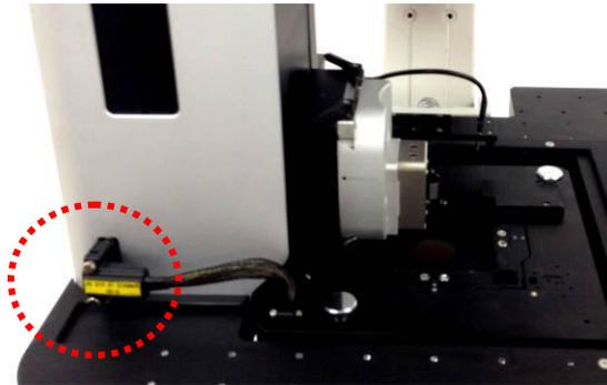
**Figure 3-12. XY Scanner Cable Connection**
