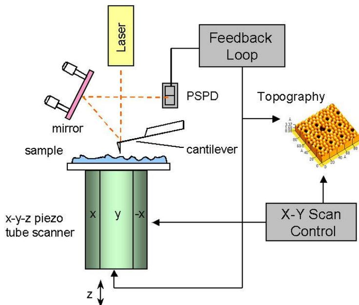
**Figure 1-1. Diagram of Conventional AFM's Scanning**
