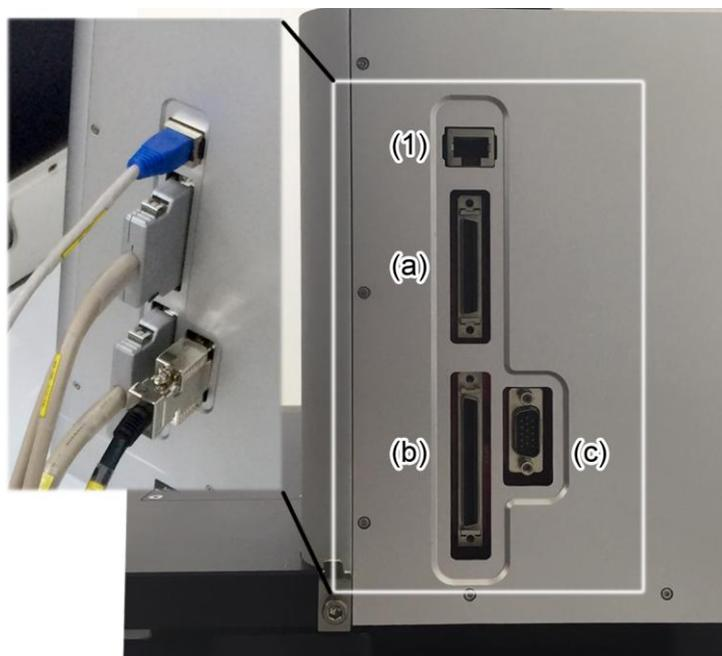
**Figure 3-11. Cabling NX12 control electronics**
