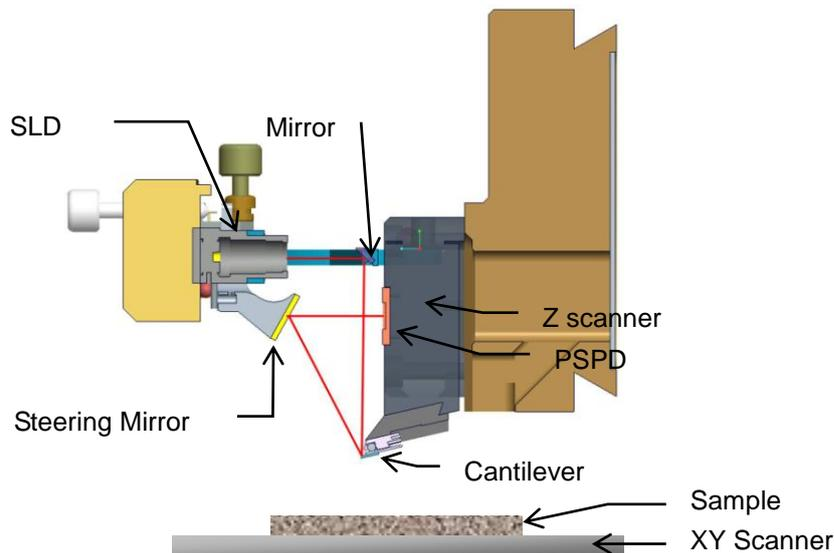
**Figure 1-3. Z Scanner Separated from XY scanner**
