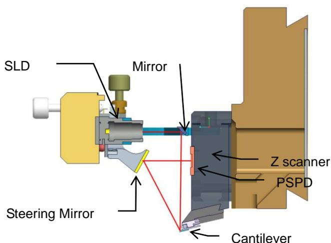
**Figure 7-5. Beam Detection**
