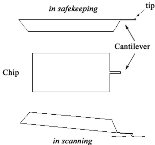
**Figure 7-8. Cantilever Chip**
