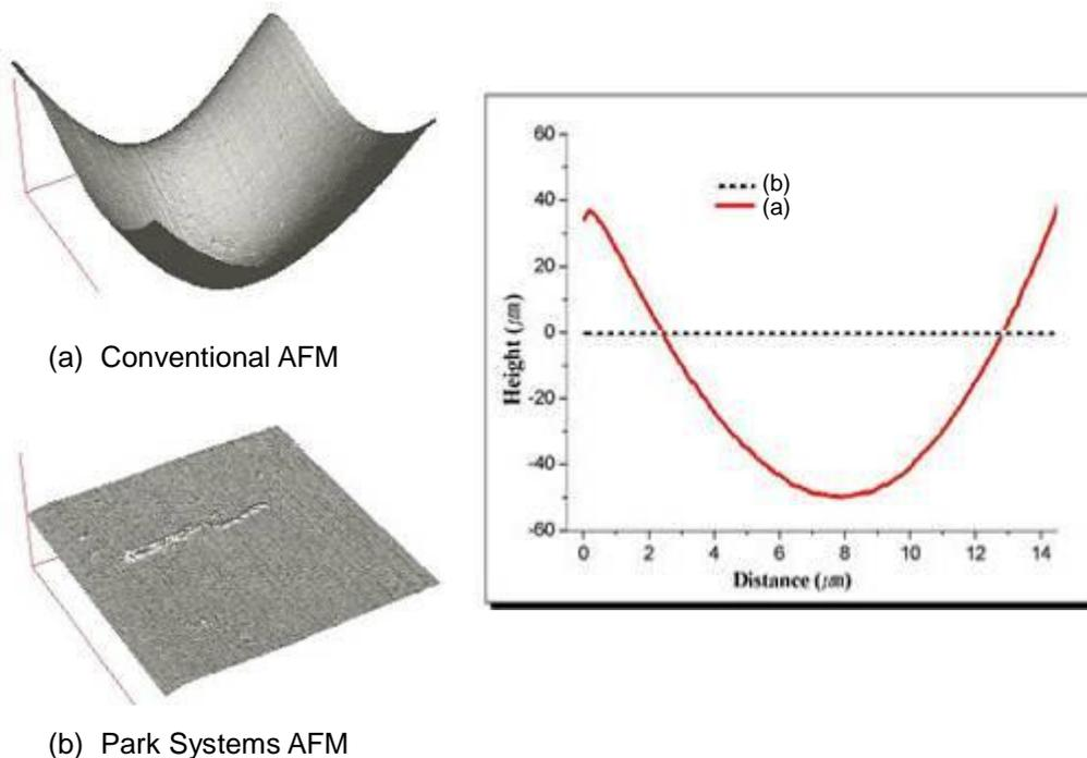
**Figure 1-4. Background Flatness Images from a Conventional AFM (a) and Park Systems AFM (b)**
