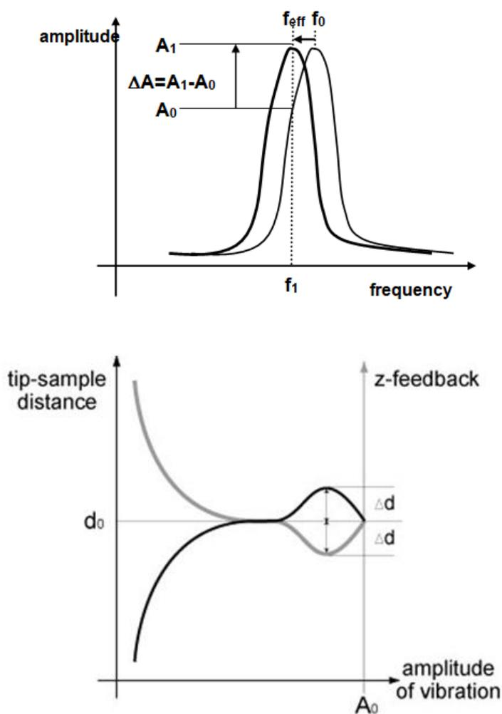
**Figure 7-37. (a) Resonant frequency shift (b) Amplitude vs. Z-feedback**
