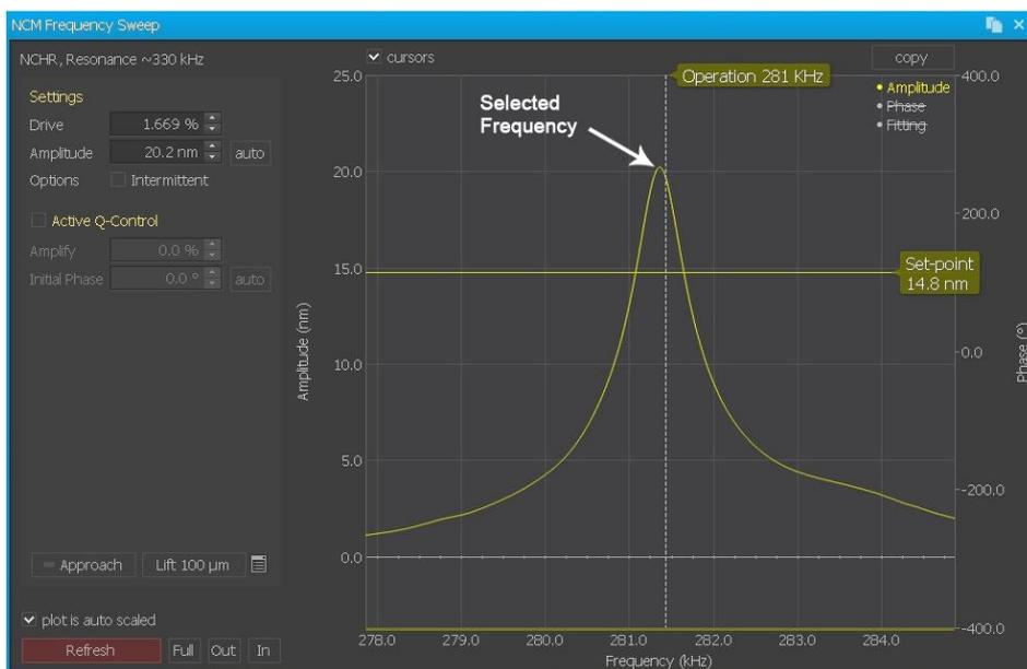
**Figure 7-39. Resonant frequency setup in Tapping mode**
