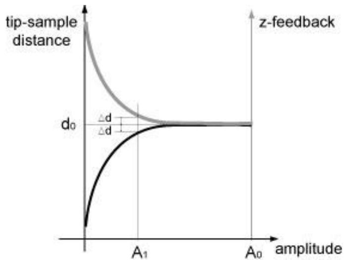
Figure 7-30. (a) Resonant frequency shift (b) Amplitude vs. z-feedback and tip-sample distance
