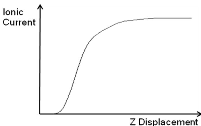
**Figure 8-17. Measured Current VS Distance Curve (DC Mode)**
