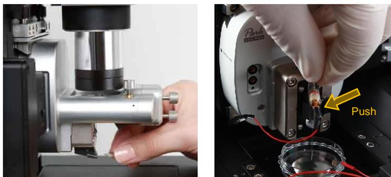
**Figure 1-7. Probe/Pipette Exchange**
