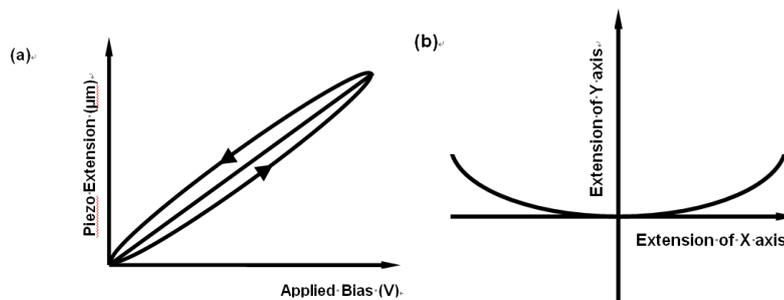
**Figure 1-2. Nonlinearity and Hysteresis (a), and Cross Coupling (b)
