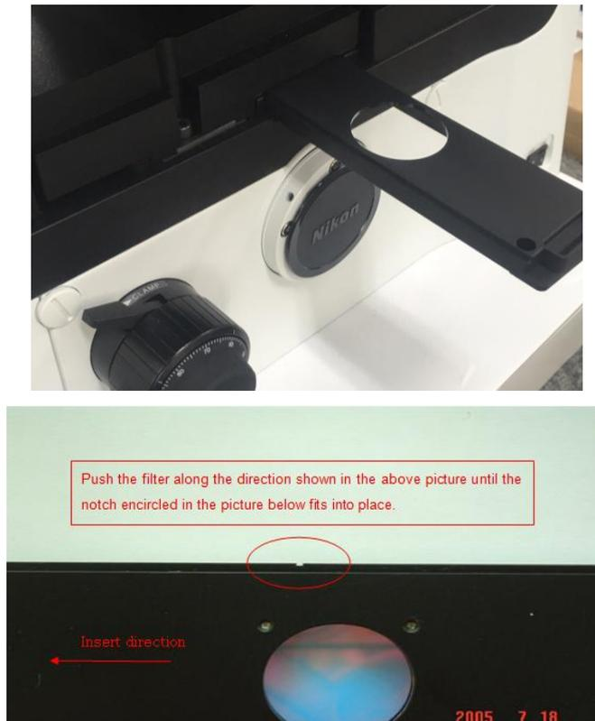
**Figure 2-14. Assemble Filter Holder**
