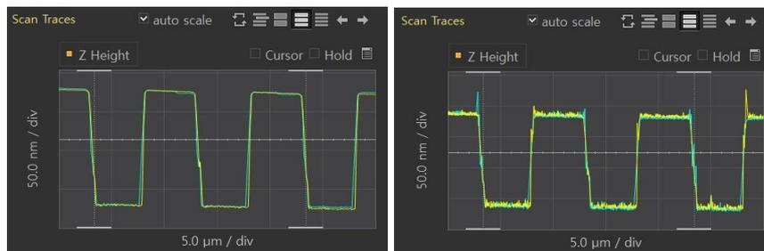
**Figure 7-35. Proper Gain (top); Noise from Excessive Gain (bottom)**
