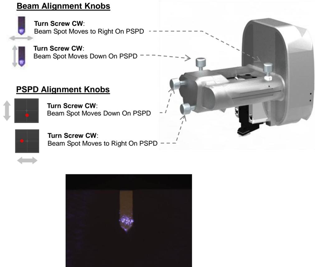
**Figure 6-7. Beam Alignment Controls**
