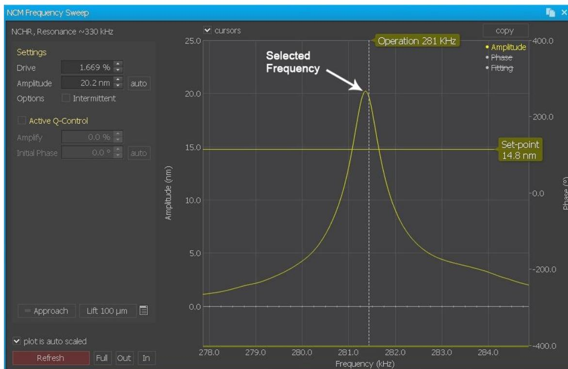
**Figure 7-31. Resonant Frequency setup in Non-Contact Mode**
