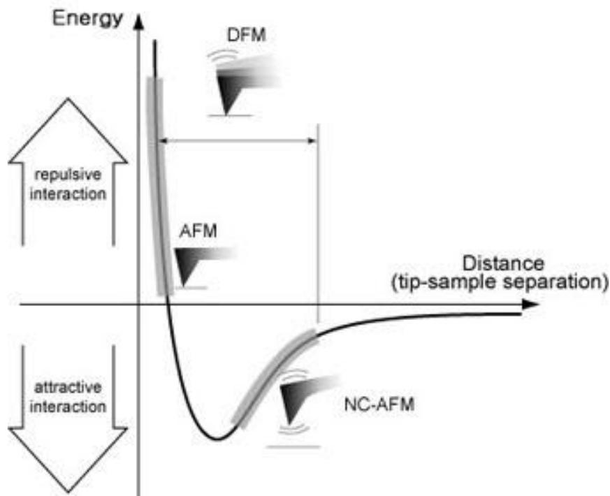
**Figure 7-20. Relation between the force and the distance between atoms**
