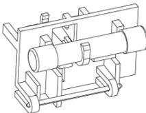
Install fuses on one side only. Do not install both AG and Metric fuses at the same time.
