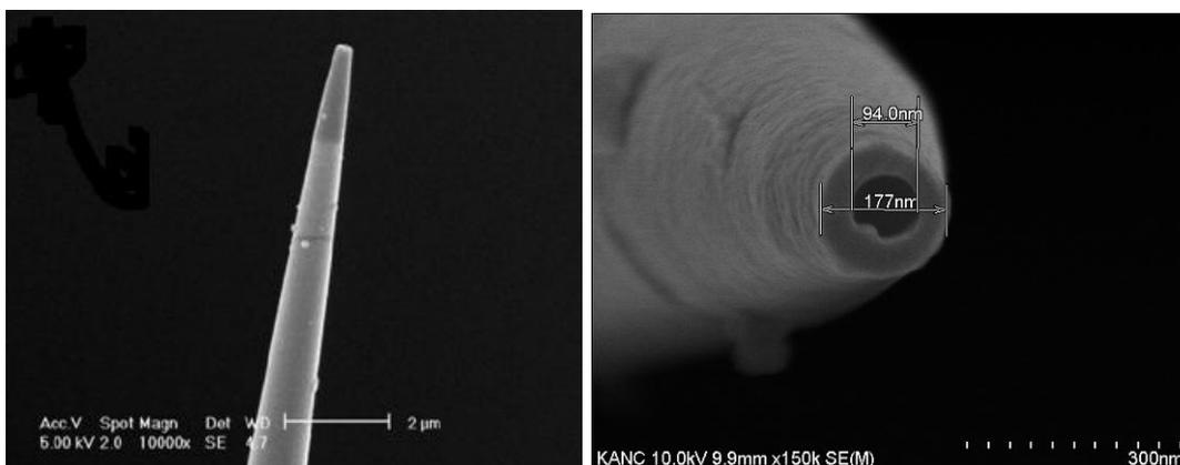
**Figure 8-3. Nano-pipette SEM Image**
