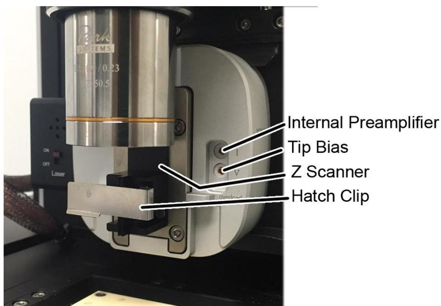
**Figure 2-3. (Top) AFM Head and (Bottom) SICM Head (Optional)**
