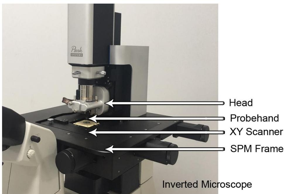
**Figure 2-2. NX12 Scanning Probe Microscope**
