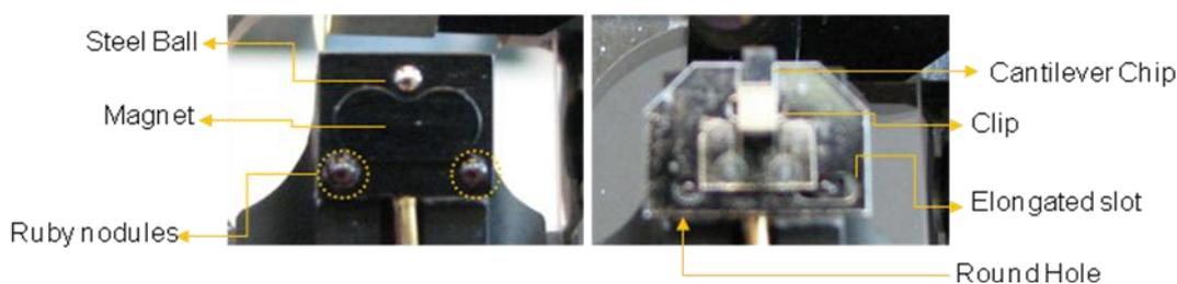
**Figure 7-3. Checking Probe Hand**
