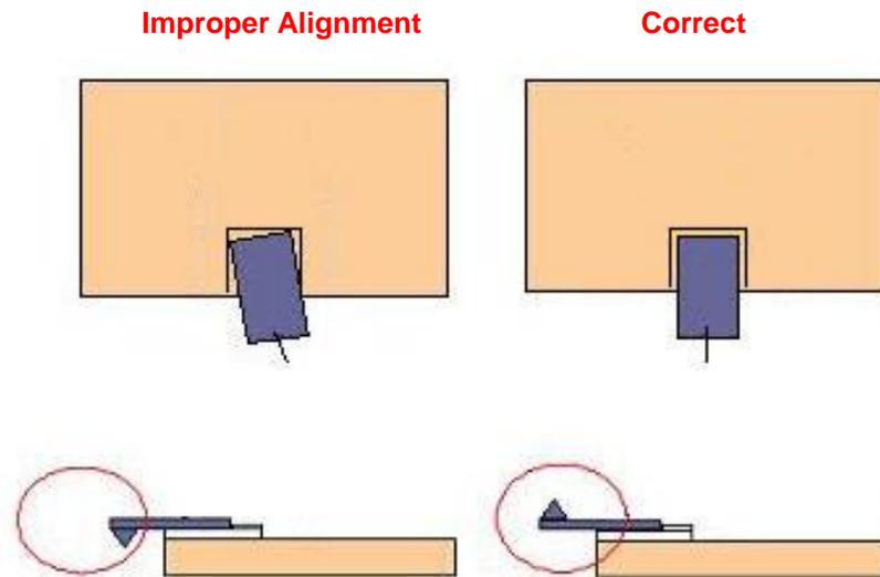
**Figure 7-14. Correct Mounting of Cantilever Chip**
