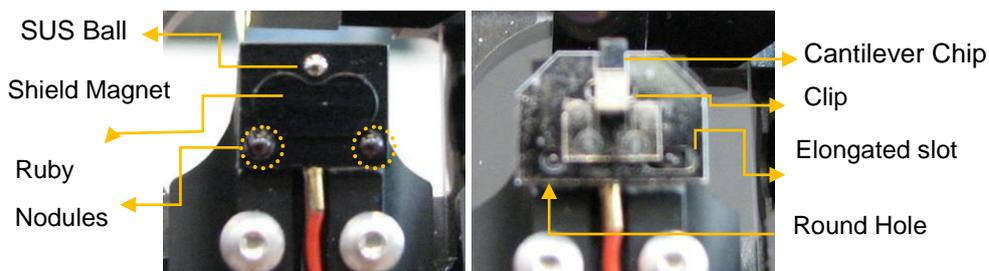
**Figure 7. Edge of Probe Hand before (left) and after (right) Chip Carrier is attached to it**
