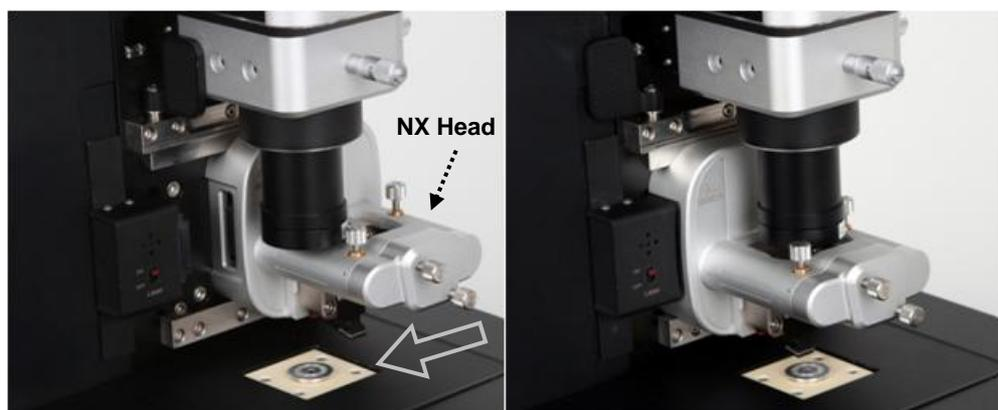
**Figure 2-5. Removing NX12 Head**
