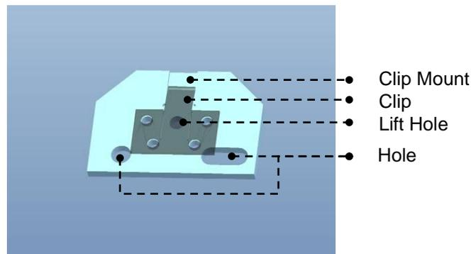
**Figure 1. Structure of Clip Type Chip Carrier**
