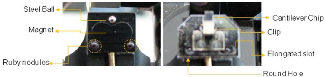
**Figure 7-16. Edge of Probe Hand before (left) and after (right) Chip Carrier is attached to it**
