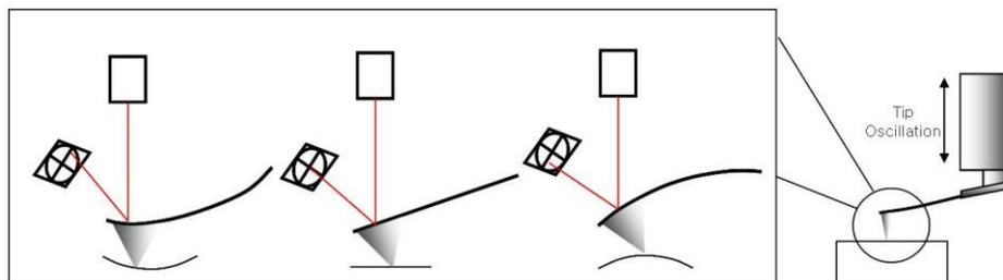
The DC deflection signal represents average deflection of the tip, which depends on the force exerted on the sample. The Z feedback loop maintains the DC deflection signal and generates a topographic image.
