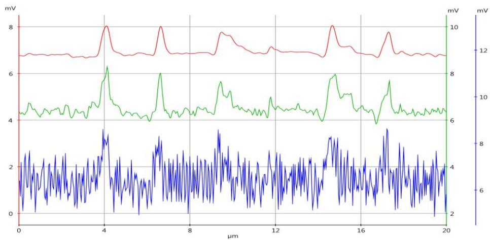
As seen above in Figure 14-31, Figure 14-32, and Figure 14-33, if the Time constant is long then image and line profile become blurry, while if the Time constant is short then image and line profile become noisy.
