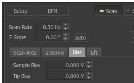
EFM tip bias is a voltage applied to the tip when the system performs the second scan to get the EFM image. It is activated when Tip-sample distance is checked. EFM tip bias is a voltage applied to the tip when the system performs the second scan of the EFM mode to get the EFM image.
