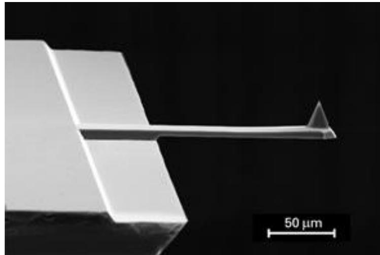
The cantilever is the part sensing the surface properties (the topographic distribution, the physical solidity, electrical properties, magnetic properties, chemical properties, etc.) by detecting the degree of deflection due to the interaction with the sample surface, and is a determining factor for image resolution.
