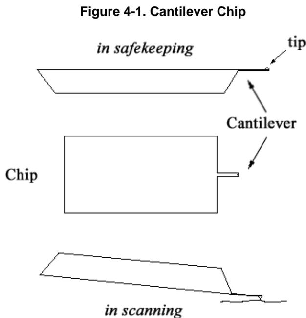
The chip, the cantilever, and the tip are made from Silicon (Si) or Silicon Nitride ( $\text{Si}_3\text{N}_4$ ), and are manufactured using macro-machining techniques.
