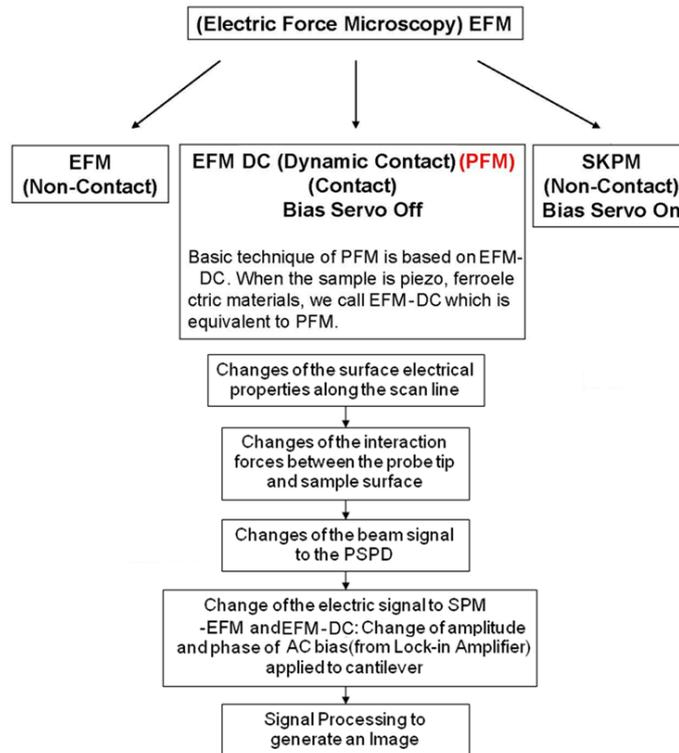
**Figure 14-1. Process of the EFM imaging**
