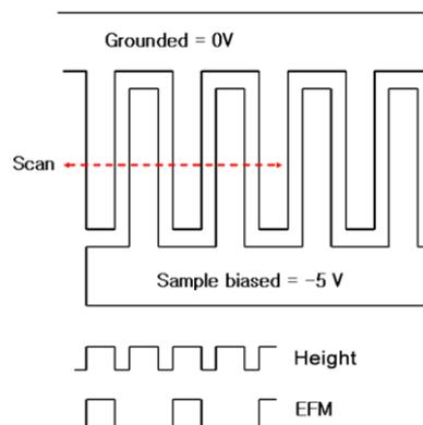
Figure 14-24. Actual Height and EFM image of the test sample
