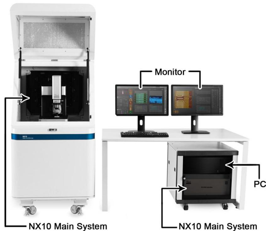
The NX10 main system is where actual measurements are made, and the NX10 control electronics control the movement of the NX10 main system according to the commands from the computer. All necessary software, including SmartScan™ (the Data Acquisition program), XEI (the Image Processing program) and the vision program, is installed on the computer.
