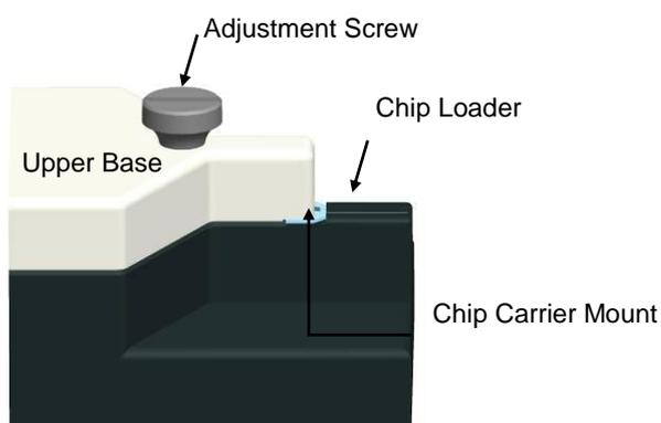
There is an adjustment screw on the upper base of the cantilever exchanger to move the upper base up or down. Turning the screw clockwise moves the upper base down and keeps the clip opened. Turning the screw counter-clockwise moves the upper base up and keeps the clip closed.
