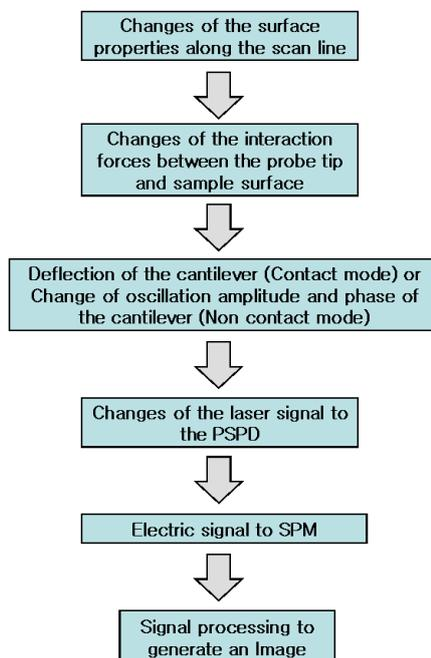
While the Van der Waals forces present in height imaging are inversely proportional to distance to the power of 7, magnetic signals are long range forces inversely proportional to the second power of distance. This is why NX SPM MFM mode scans a sample twice, in order to separate the signals. Height is measured within a range where Van der Waals forces are dominant, and then the tip is moved further away from the sample in order to measure the effects of magnetic forces.
