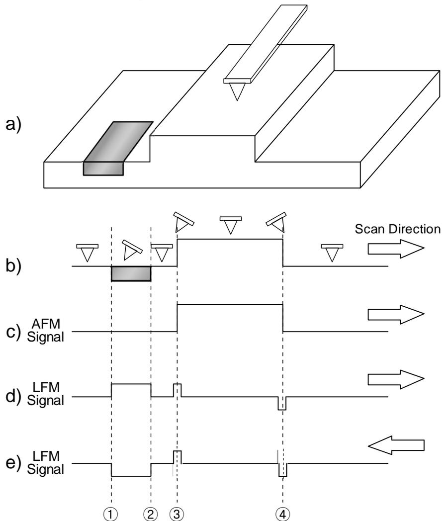
Figure 7-2 (a) shows a surface structure with a centrally located step with low, smooth
