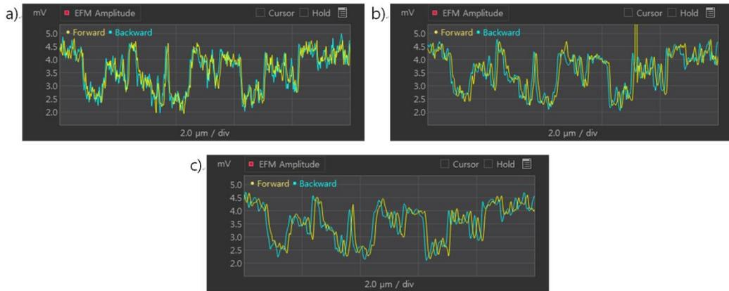
**Figure 14-32. EFM Amplitude Image according to Time constant; Time constant = a) 10ms, b) 5ms, c) 1ms**
