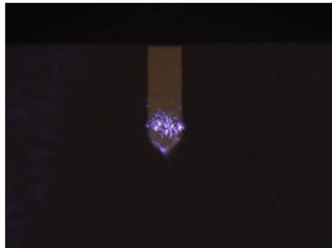
Figure 1-6 shows the cantilever with the SLD beam focused on it, as it is displayed on the vision software. Since the CCD camera is aligned directly with the cantilever with nothing blocking its view, it is very convenient to focus on or to observe the sample while moving the camera up and down. This view also provides superb quality for an optical microscope.
