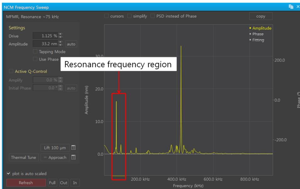
**Figure 12-14. PPP-MFMR NCM Frequency Sweep data**
