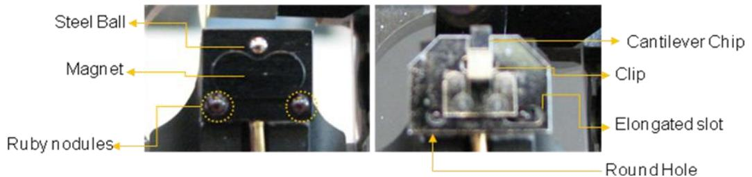
There are two holes in a chip carrier; a round hole and an elongated slot. When you overlay the two ruby nodules located on the end of the probe arm with these holes, the cantilever chip will be attached into place by a magnet, and the position of the cantilever will be firmly fixed in one position.
