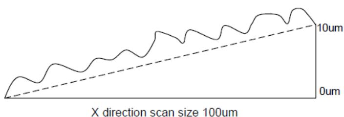
To calibrate the Z scanner, image a standard sample with a known step height and enter the measured and known (expected) heights into the calibration setup interface. A summary of the parameters for Z scanner calibration can be found in the table below. For more information about scanner calibration, please refer to the NX User's Manual.
