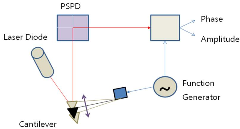
When the cantilever is vibrated at the resonance frequency, a +90 degree phase difference between the driving signal (green) and output signal (yellow, VERTICAL (AC) signal) occurs. Please see Figure 11-2.
