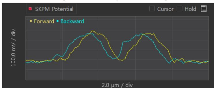
Figure 14-40-a displays a noisy line profile resulting from a large Tip bias servo gain value and Figure 14-40-c displays a blurry line profile resulting from a small Tip bias servo gain value. Adjust the Tip bias servo gain value to minimize line profile noise and synchronize forward/backward lines.
