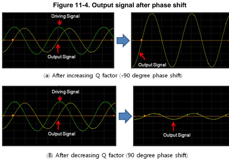
After passing through the phase shifter, the signal can be amplified again when given an appropriate gain. This additional feedback circuit is called a “Gain Amplifier”. Figure 11-5 shows a schematic diagram of Non Contact mode with Q Control. The output signal, the AC signal from PSPD, passes through the Phase Shifter and Gain Amplifier and is then sent to the Adder. Finally, it is added to the driving signal for cantilever motion.
