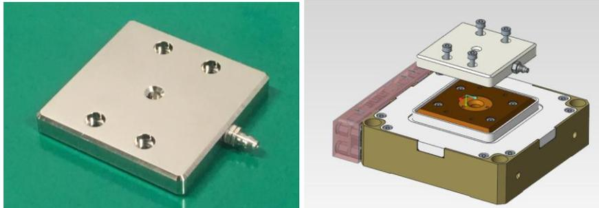
Check the vibration noise by applying a sample Bias to the structure attached to the existing sample chamber. The vacuum sample chuck can be mounted on the NX10 sample chuck.
