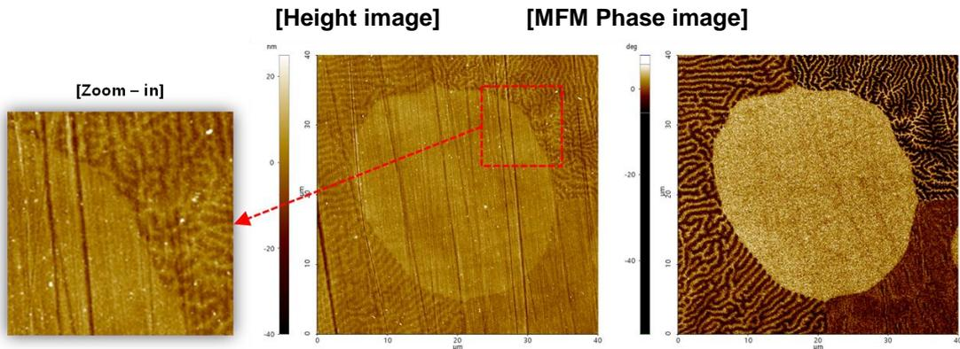
Figure 12-15. Example of MFM signal interference in Height image
