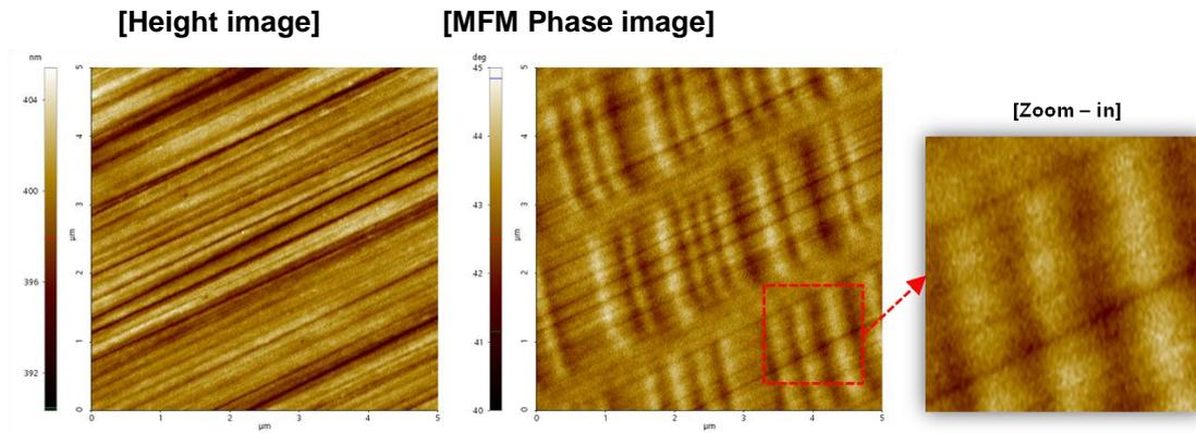
Figure 12-17. Example of Height signal interference in MFM image
