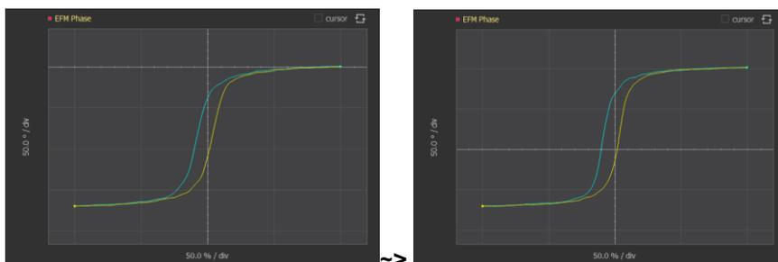
EFM phase is used for KPFM feedback. This value includes polarity of sample and Y offset from system in fact. Therefore, we need to set the signal above by adjusting phase shift on the Lock-in Amplifier in order to distinguish the polarity of the sample potential.
