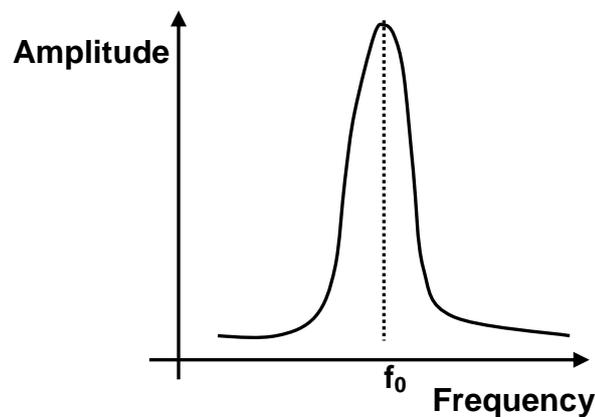
On the other hand, the spring constant affects the resonant frequency ( $f_0$ ) of the cantilever, and the relation between the spring constant ( $k_0$ ) in free space and the resonant frequency ( $f_0$ ) is as in Equation (2).
