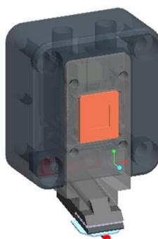
The NX10's Z scanner is separated from the X-Y scanner. This independence provides the user with several operational advantages.
