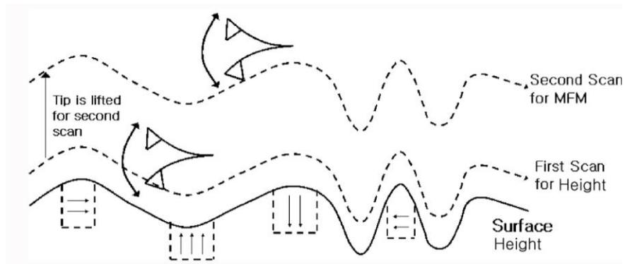
Figure 12-3 Obtained signals in MFM mode
