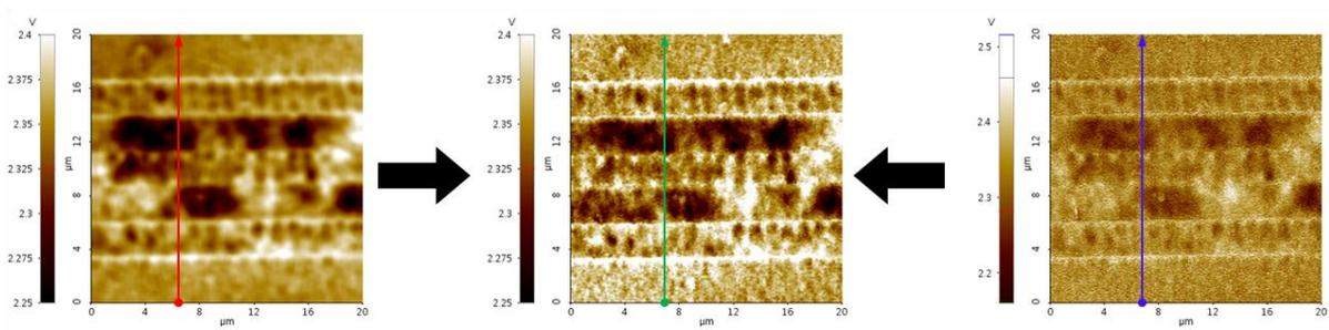
Figure 14-38; a) Tip bias servo gain=0.1, b) Tip bias servo gain=0.3, c) Tip bias servo gain=0.5
