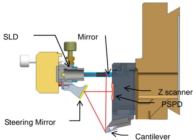
The cantilever and the PSPD move together with the Z scanner while the SLD beam, a steering mirror and a fixed mirror are fixed relative to the scanner frame. The SLD beam, positioned in front of the Z scanner, is aimed at a fixed mirror that is situated above the cantilever. The mirror reflects the SLD beam downward and onto the back surface of the cantilever. The SLD beam will always hit the same spot on the cantilever
