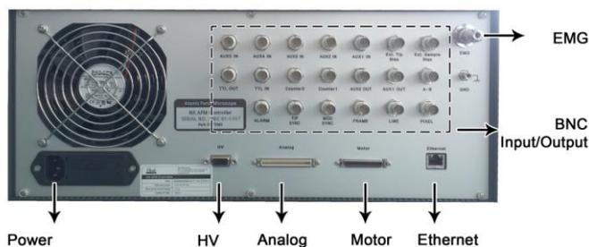
In order to maintain fast, effective communication between the computer and the NX10 main system, an Ethernet connection is used. The DSP contained in the NX10 Control Electronics is the 9600MMACS.
