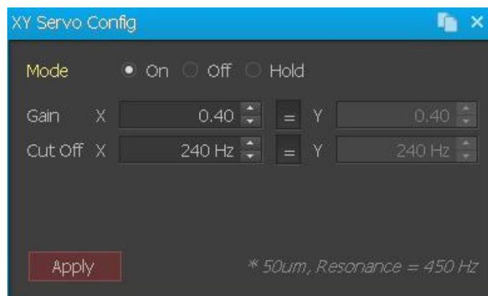
In general, piezoelectric materials display nonlinear behavior in response to an applied voltage. Therefore, the scanner, which is made of a piezoelectric material, displays nonlinearity and hysteresis (Refer to Chapter 1). When the scanner's range of motion increases, nonlinearity and hysteresis can be calibrated by means of hardware corrections.
