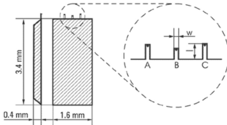
Table 6-1 shows the specification for the three cantilevers in the NSC36 series.
