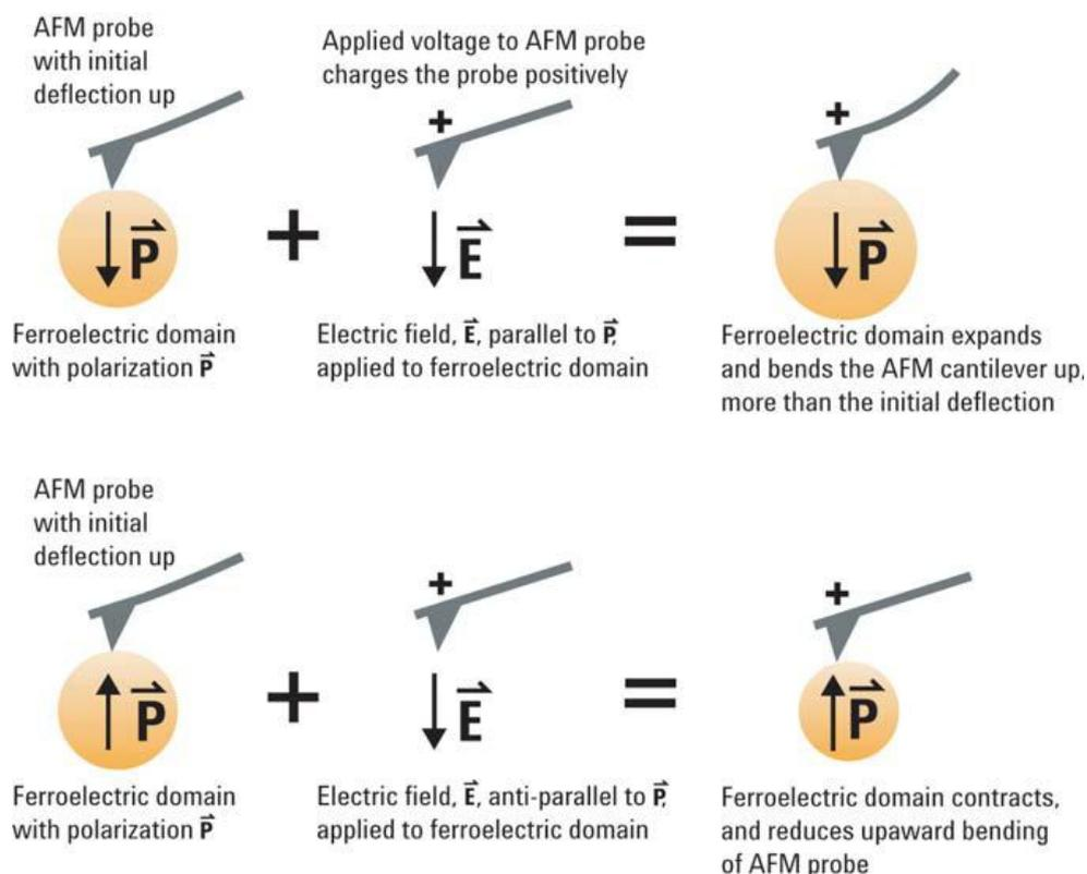
If the applied voltage contains a small AC component, the inverted piezoelectric response from the sample would result in sample surface oscillation in the same frequency as the applied AC voltage. In the case that the sample is an ideal piezoelectric crystal, its polarization  $\vec{P}$  would be related to applied mechanical stress  $\vec{s}$  by the following equation:
