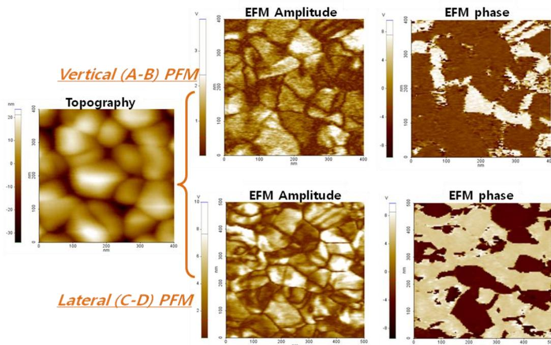
In most of the real cases, the studied sample contains random-oriented polycrystalline grain structure, often with non-zero lateral components in its piezoelectric tensor. In this case, the detected vertical PFM signal is no longer only proportional to  $d_{33}$ , but also dependent on the  $d_{31}$  and  $d_{15}$  components. E.g., the vertical PFM amplitude would no longer be  $\Delta Z_0 = d_{33} V_0$ ; instead, it would take the form
