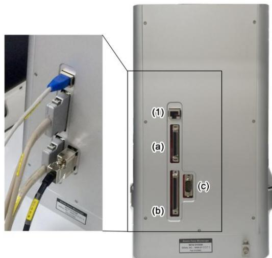
**Figure 3-10. Cabling NX10 control electronics**
