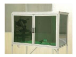
The Laser safety cabinet serves two purposes in one. It protects the instrument from dust and air convection at the same time protecting the user from scattered laser light. The acrylic glass is colored to absorb the laser wavelength, still allowing visual control of the instrument.
