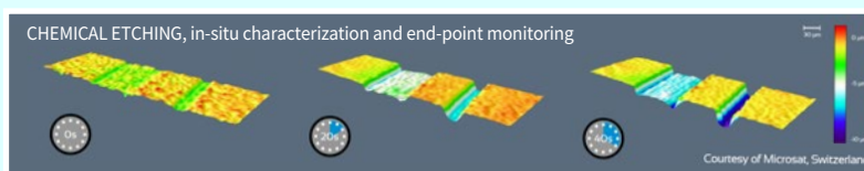
In situ monitoring of electrochemical etching of 20 µm and 100 µm trenches using a glass corrected 20x objective.
