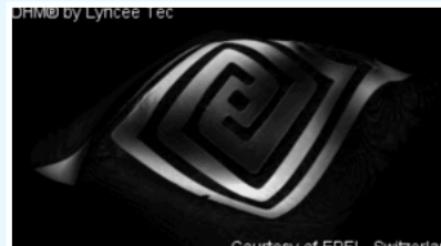
Thermal deformation of a Micro Hot Plate @ 800°C 5× objective (NA 0.12). FOV 1.2 mm × 1.2 mm.
